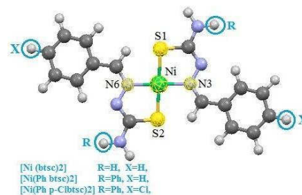
Fig. 1 : Optimized structures of tsc complexes.
